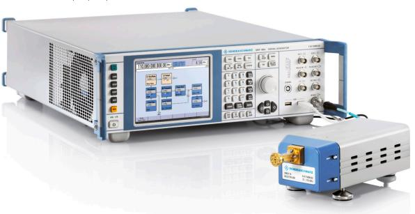
Test setup containing the R&S<sup>®</sup>SMF100A microwave signal generator and the R&S<sup>®</sup>SMZ110 frequency multiplier.
